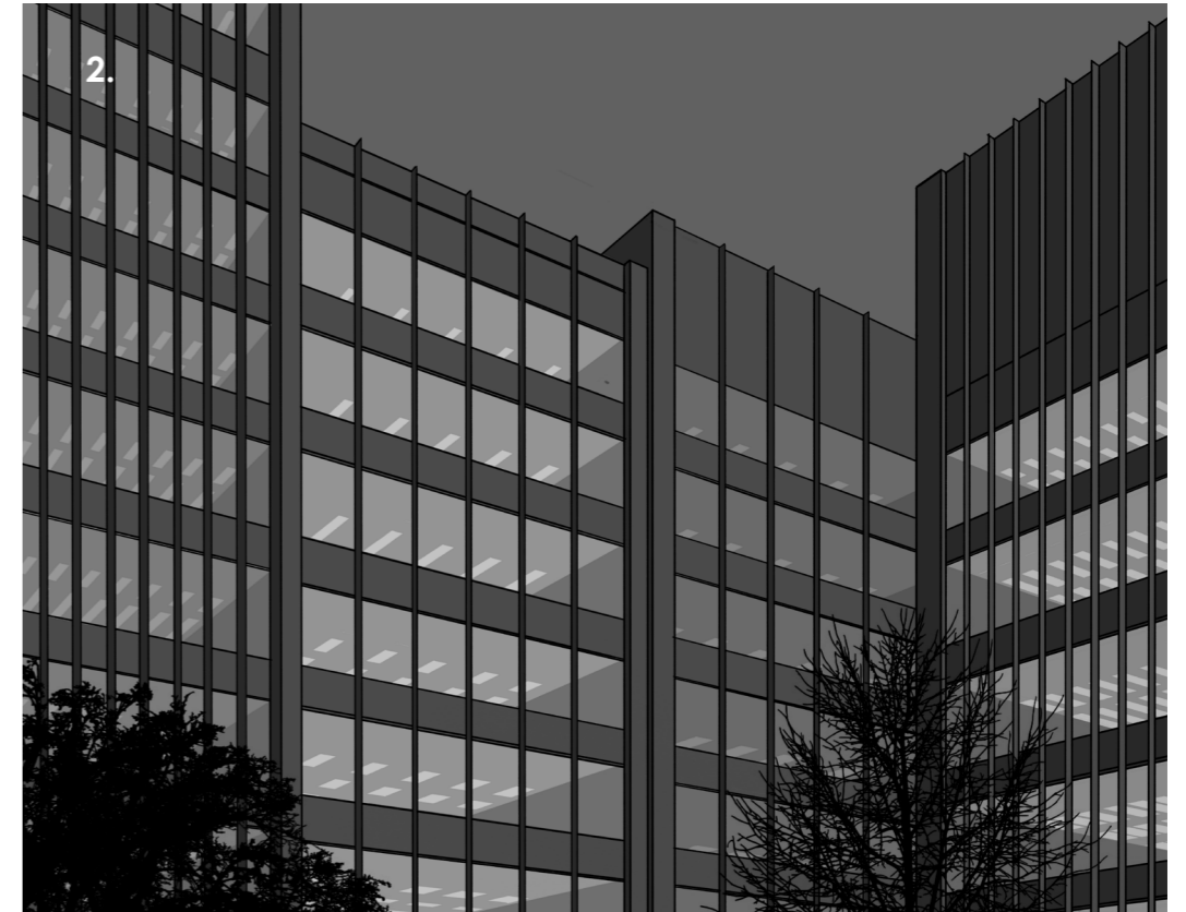
2. Blinds, coatings, frit patterns and other facade design techniques can help reduce the visibility of interior lighting at night while occupants can still perform their tasks. All developments should switch off the internal lighting when the building is not occupied.
