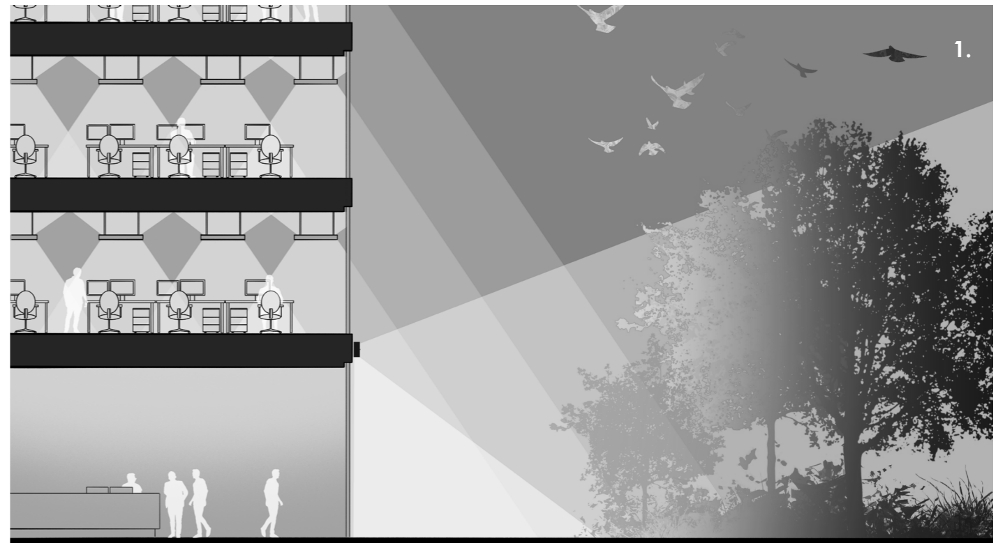
1. Glazed facades without treatment and external lighting with insufficient optical control can cause light trespass into green areas spaces and potentially create bird strike.
